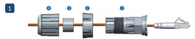
Follow the order from 4 to 1 and put components through cable accordingly, no need to assemble here.
