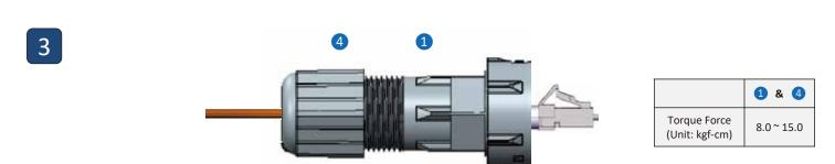
Then assemble  $3 \rightarrow 1$ ,  $4 \rightarrow 1$ ) and follow the torque force accordingly.
