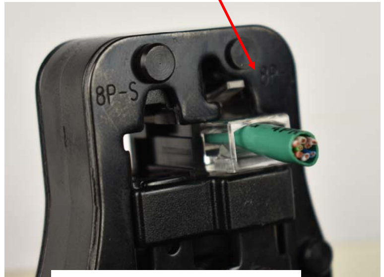
Crimping the Long Body RJ45
