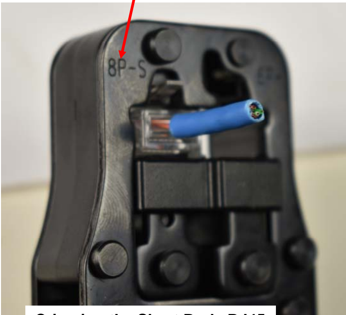
Crimping the Short Body RJ45
