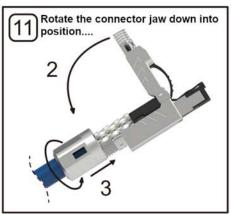
....and snap it closed. Screw the nut up tight onto the connector body to complete the assembly.
