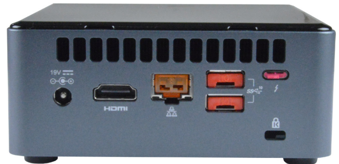
VPI's selection of port blockers inserted into connectors of a computer – RJ45, USB Type A, USB Type C
