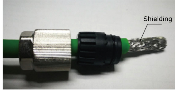
Step 2: Strip the cable jacket back 1"
