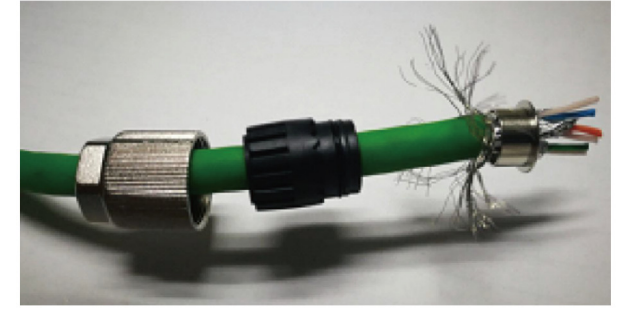
Step 3: Pull back the shielding and place the shielding tube onto the cable
