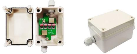
SP-POE-WTP is a high quality surge protection device designed to protect outdoor POE/Network equipment from lightning. The product is enclosed in a IP66 outdoor housing which could be easily mounted on a wall or pole. It supports data transmission up to 1 Gigabit and a POE device up to 90W.
