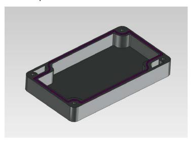
B) Align the cover with the base. Insert four screws (provided) into the corner holes. Tighten the screws evenly to 7inch-lb torque. **DO NOT OVERTIGHTEN**.
