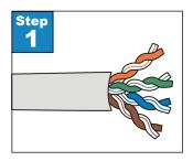
**Step 1.** Carefully strip the jacketing from the cable to expose 1" of the insulated wire conductors. Do not remove any insulation from the conductors.
