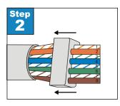
**Step 2.** Untwist the pairs to within 1/8" of the jacket. Arrange the wires according to TIA/ EIA 568A & 568B standards. Flatten and align the wires. Make one straight cut across all the conductors, removing approximately ½". Insert wires into loading bar. Trim excess wires.
