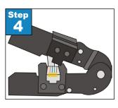
**Step 4.** Insert the plug into a crimp tool. Firmly squeeze the handles to set the contacts and secure the cable.
