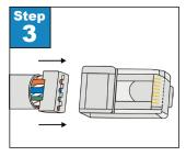
**Step 3.** Insert prepared cable into plug.
