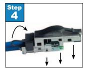
**Step 4.** Finally align the plug with the appropriate slots of the IDC and press down firmly (with either using your fingers or a Parallel Crimp Tool) until you hear it snap together. Apply the strain relief cover over top of the cable and into the designated slots located on the sides of the IDC.
