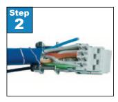
**Step 2.** Flatten and align the wires appropriately to be seated within the plug.
