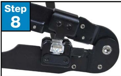
**Step 8.** Insert the plug into a crimp tool aligned to the slotted jaw. Firmly squeeze the handles to set the contacts.
