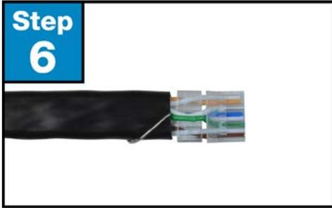
**Step 6.** Flatten and align the wires. Make one straight cut across all the conductors, removing approximately 1/2". Insert wires into horizontal loading bar. Trim excess wires.
