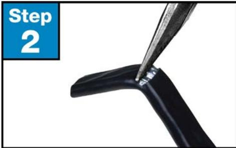
**Step 2.** Flex the cable where you scored it and use needle nose pliers to peel off the jacket. Use wire cutters to trim any excess that does not peel off.
