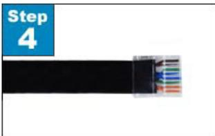
**Step 4.** Untwist the pairs to within 1/8" of the jacket. Arrange the wires according to TIA/EIA 568A or 568B standards. Flatten and align the wires. Make one straight cut across all the conductors, removing approximately 1/2". Insert wires into loading bar. Trim excess wires.
