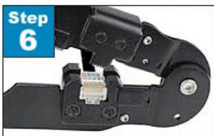
**Step 6.** Insert the plug into a crimp tool aligned to the slotted jaw. Firmly squeeze the handles to set the contacts.
