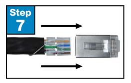
**Step 7.** Insert prepared cable into plug.
