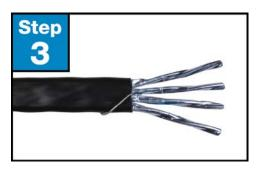
**Step 3.** Expose 1" of the shielded wire conductors. Wrap the drain wire around the cable.
