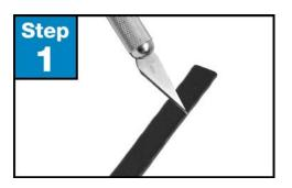
**Step 1.** Lay the end of your cable on a flat surface. Using an x-acto knife, very carefully score the jacket across the cable 1" from the end.
