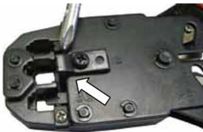
Image 3. Remove to prevent damage to the plug.
